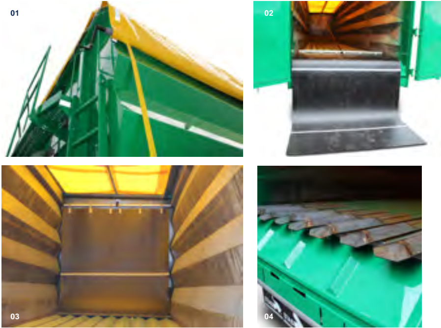
01 manuelle Plane 02 en 03 CleanSweep 04 V-Floor Keith Walking Floor
